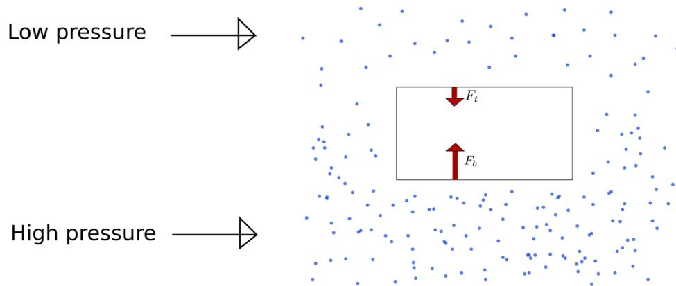
FIGURE 2.2. The difference of forces on the top and bottom surfaces is the resultant buoyancy force.
